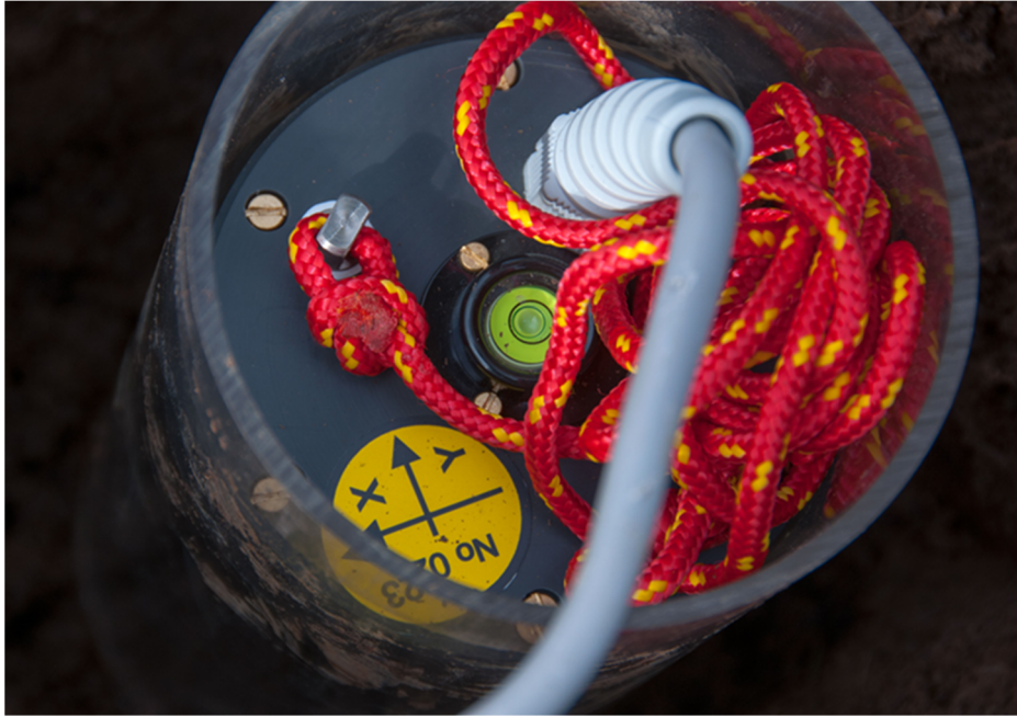
Figure 3: A LEMI-039 magnetometer housed in a clear acrylic protection housing. Note that the cap has been temporarily removed from the housing for clear display of the bubble level and magnetometer.
