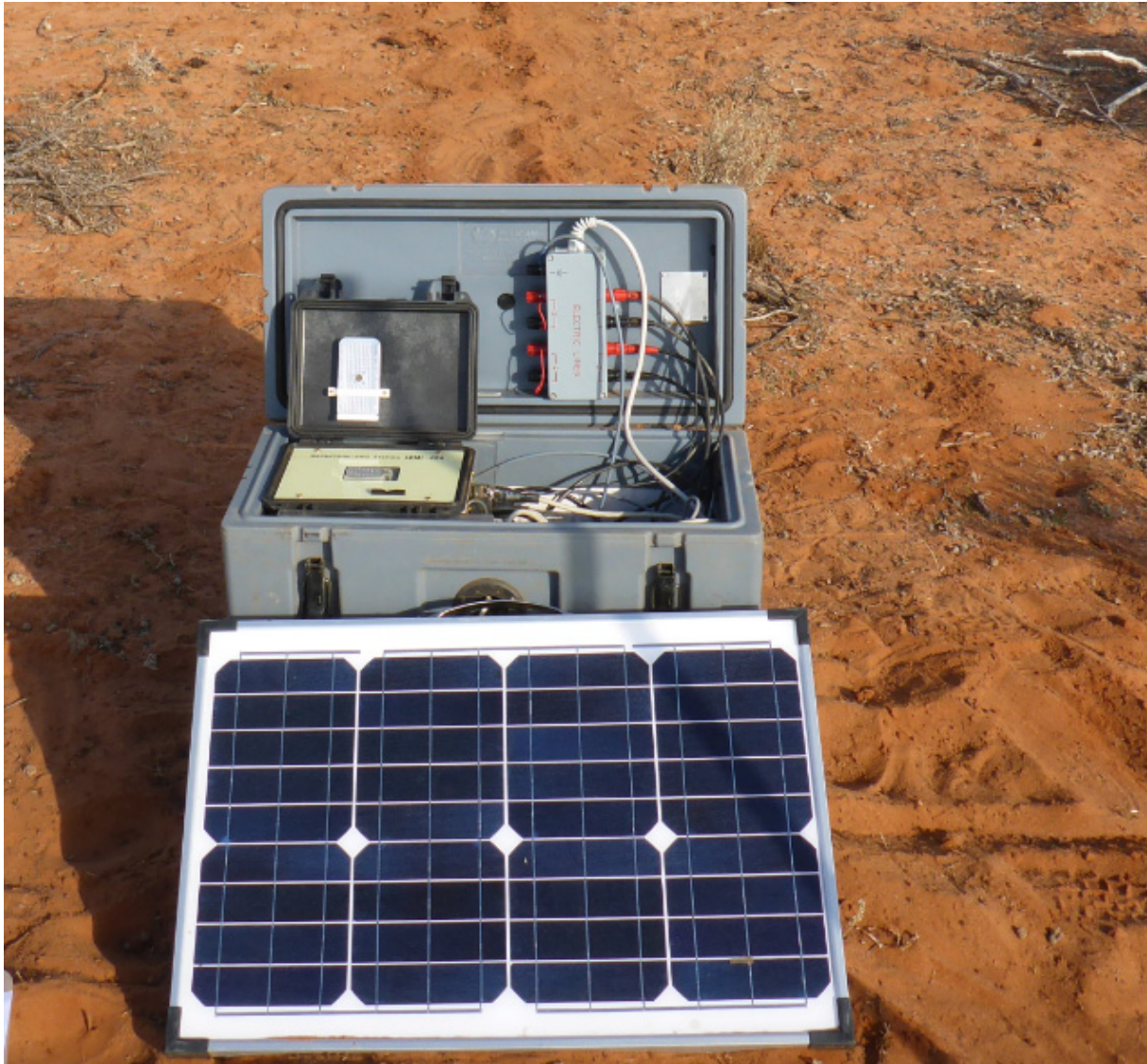
Figure 2: Geoscience Australia's typical LEMI acquisition system. The weatherproof plastic case contains an acquisition unit, an electric line junction box, a GPS antenna and a battery. A solar panel is attached to the case to charge the battery.
